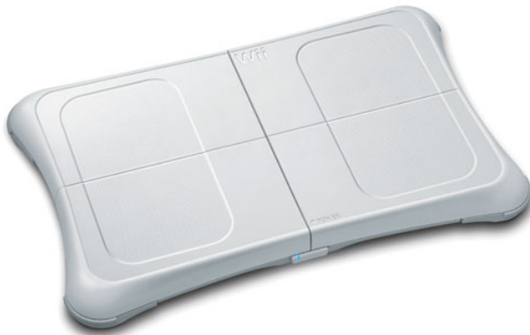
(b) Force platform (Wii Balance Board ©)
